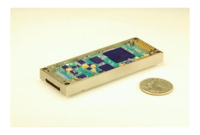
The MI\_BASE3 module with a Micro Series power supply module connected forms a base data acquisition unit for a standalone or distributed PCM system.
