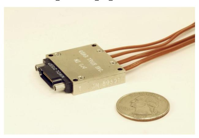
The MI\_CJ4 uses 4 digital thermometers, and outputs the four digital cold junction temperatures in SPI format, offering the following advantages:
